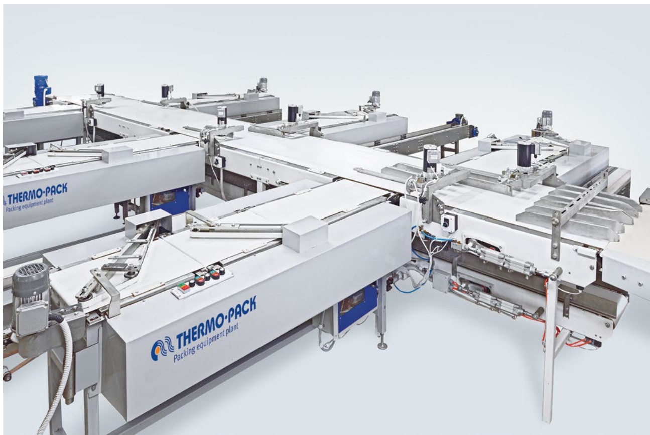
4.01 Distributing conveyor together with feeding conveyor and wrapping units
