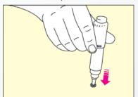
Place the lancet protective cap on a hard surface, then push the used lancet tip into the lancet protective cap which was removed earlier.
